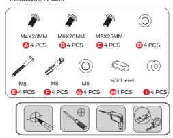
Tools required: pencil, Philips head screwdriver, power drill, measuring tape
